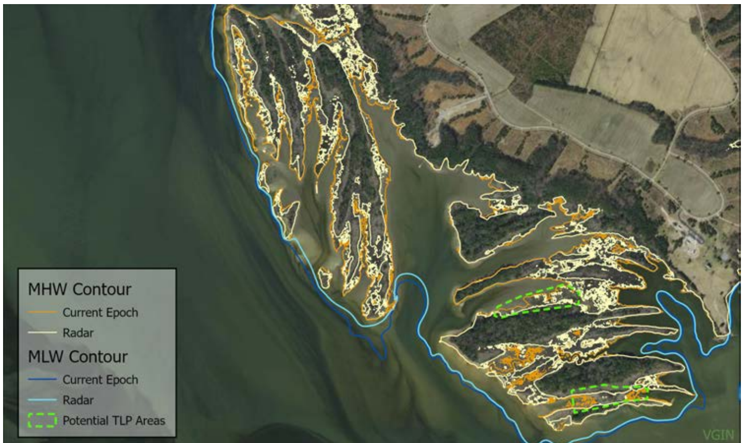
Figure 13: Elevation contours from the USGS CoNED project. Current Epoch contours are from the NOAA COOPs station at Yorktown from 1980-2001. Radar contours use calculated tidal datums from the radar gauge on site. Green squares highlight areas identified for potential Thin Layer Placement (TLP).
