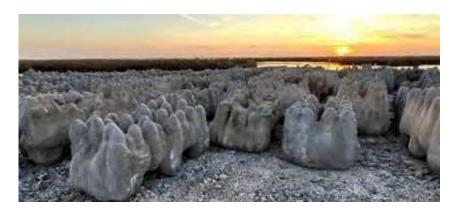
**Oyster Catcher (SANDBAR):** reef substrates that are a composite derived from cement infusion of plant-based cloths. They can be molded into different shapes such as tables, pretzels and pillows that can be stacked and tiered to increase settlement surface area. Textured surfaces encourage oyster settlement and seeding is possible.
