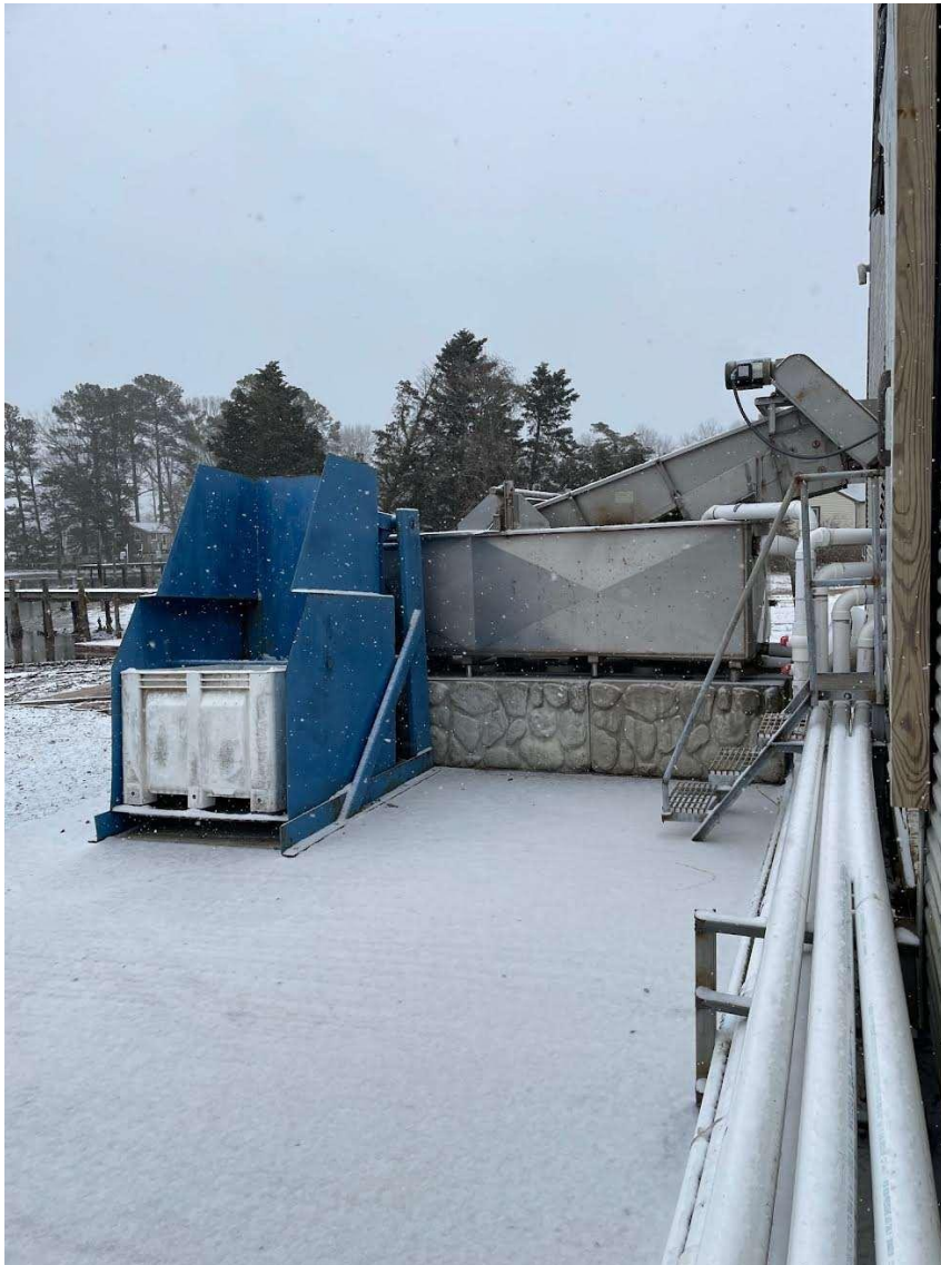
This picture shows a hydraulic pallet tote dumper and a stainless hopper feed conveyor.
