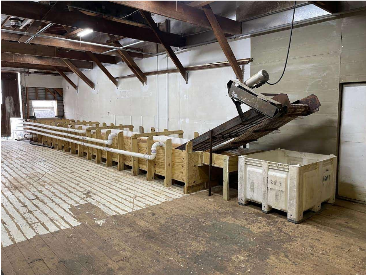
This picture shows the final design variation of our brine tank and conveyor system. This design is the prototype prior to stainless construction.
