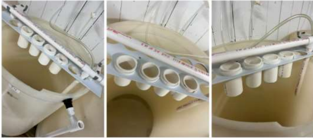
Figure 2. Photo of the downweller tank setup used in this project. Each tank had a capacity of 200 liters, and each cup measured 5 cm in diameter, fitted with a 500 \mu\text{m} mesh screen at the bottom.
